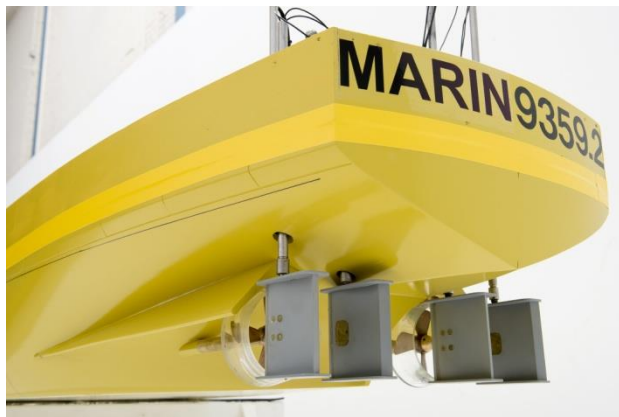
Figure 4. Propeller and rudder arrangement for the twin screw variant: ship model
