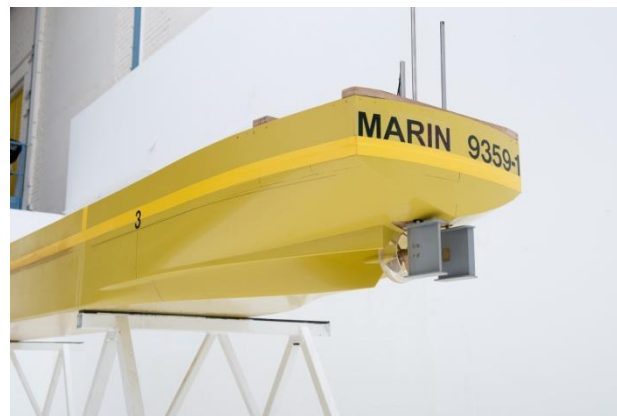
Figure 2. Propeller and rudder arrangement for the single screw variant: ship model
