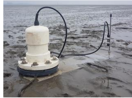
Figure 1. The pressure sensors (PTX 1830) used to collect data of ship passages
