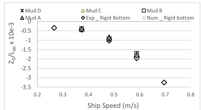
Figure 11. Ship sinkage as a function of the mud properties for an effective UKC of +10%. Z_G is the sinkage at the midship
