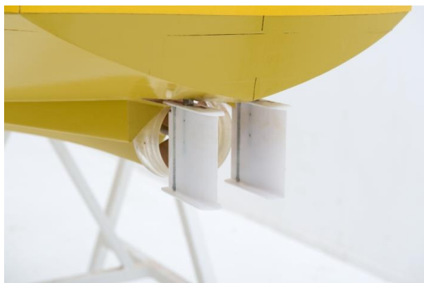
Figure 6. Propeller rudder arrangement for the single screw arrangement with a twin NACA rudder: ship model
