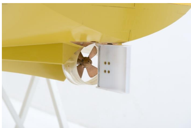
Figure 5. Propeller rudder arrangement for the single screw arrangement with a single fishtail rudder: ship model
