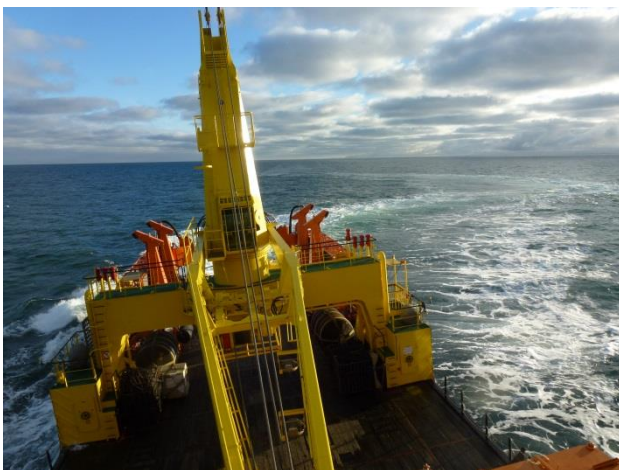
Figure 5. Zig-Zag Manoeuvre in shallow water with Multipurpose Vessel MELLUM (Photo: BAW)
