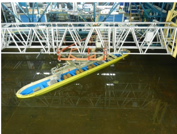
Figure 8. Set-up of model test with -40^\circ drift angle (bow to portside)
